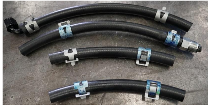
4Runner Hoses with factory clamps installed.
