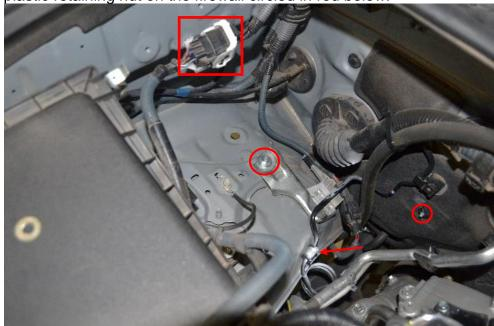
3. Installing the Dual Battery Kit. Slide the Vertical Support in between the loosened brake clamp and align the rear of the bracket onto the stud protruding from the firewall. Thread (1) M6 S.S. Locknut and (1) 1/4" S.S. Washer onto the stud protruding from the firewall. Begin tightening the factory brake line bolt.
