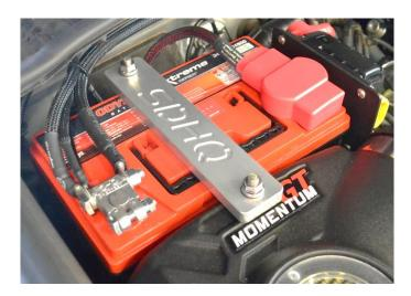
**13.** With the batteries in place, the install of the SDHQ Dual Battery Kit is complete. Now, the battery will need to be wired. If the SDHQ Dual Battery Wiring Kit (SDHQ-50-3002-U1) was purchased, begin those Install Instructions.
