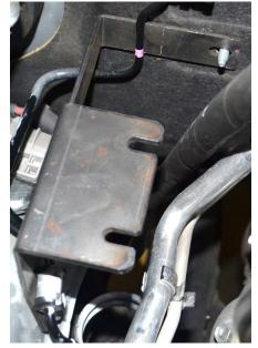
**4.** Align the Rear Upright Support over the rear stud on the wheel well as pictured. Secure the Rear Upright Support using (1) M8 S.S. Nylock Nut and (1) 5/16" S.S. Washer. Tighten this nut until the Rear Upright Support only has a little bit of room to rotate. Relocate the harness that was on the inner fender to the Rear upright Support as circled in red below right. This harness will run underneath the <u>Dual Battery Mount</u>.
