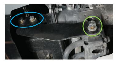
**3.** Next remove the center most frame horn bolt using a 14mm socket, these bolts will not be reused.
