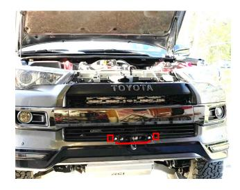
11. If you have a SR5 model, move on to step 12. Place the outer plastic back on the bumper temporarily and use the cut opening to trace onto the bumper. Remove the outer plastic and cut the bumper to match your outline. It will help to make this opening slightly larger than your traced outline since this part of the bumper is hidden.
