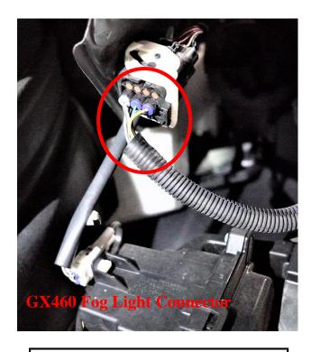
Flip up the white portion of the 6-pin connector and then you can release the plug. All the bumpers connections are made through this plug, no need to disconnect anything else individually.
