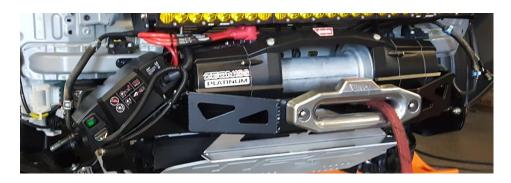
**16.** Make sure all of the winch mount hardware is tight. Reinstall the factory bumper skin in the reverse order of disassembly. Use the provided  $\frac{1}{4}$ " bolts, washers, and lock nuts to mount the passenger side lower bumper to the factory inner fender, and bottom of the bumper to the Lower Bumper Bracket. Reverse Steps 3-1 to finish assembling your vehicle. Enjoy your SDHQ Built Hidden Winch Mount!
