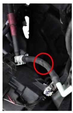
The bumper side of this connection will let fluid escape, have a small drip pan ready. Crimp the washer line temporarily on the washer bottle side to avoid losing all the fluid from the reservoir.
