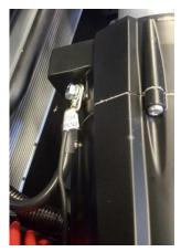
9. Wire your winch according to the manufactures recommendations. If using Warn Zeon or Evo, refer to the Zeon controller relocation and wiring kit instructions, PN: 54-1660-G5, for wiring and mounting instructions (sold separately). GX 460/470 owners can proceed to Step 1 in their respective install instructions.
