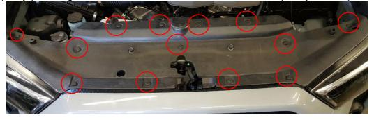
2. Then remove the (2) clips and (3) 10mm bolt holding the top of the grille.
