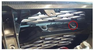
**4. Installing the mounts and light bar.** Utilizing the holes you just removed the body clips from, Insert the provided 5/16" button head screws with washers through the provided brackets into the holes in the grill support and install washers and lock nuts on the underside of the grille support. Tighten down screws just enough to lightly hold in place but still allow adjustment in the slot.
