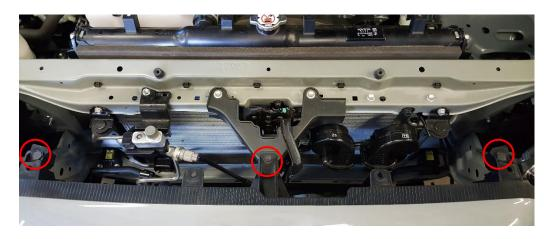
3. Finally, remove the (4) clips holding the upper section of the back of the grille on.
