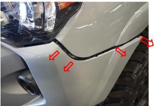
**6.** Remove plastic side air deflectors and set aside, each side is held in by a single body clip through the side and clipped into the radiator support. After removing the body clip, a good tug will unclip the deflector from the radiator support. These will not be going back on.
