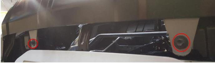
**5.** Next remove the (3) 10mm bolts on each side of the bumper that connect to the inner fenders. The top rear corner of the bumper where it meets the fender needs to be pulled straight out away from the fender, which will require prying it over the plastic threads. Then gently pull the outer section of the bumper forward, it is clipped in under the fender and light. The entire front bumper and grill assembly should come off.
