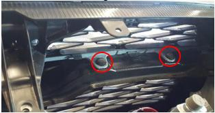
**4.** Unplug your factory fog lamps. Remove the 10mm bolts holding the front of your inner fenders to the bottom of the bumper, and the lower center section of the bottom of the bumper.
