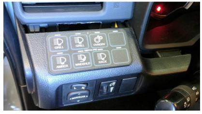
2. Disconnect the all switches and fully remove the panel. The switches will need to be removed as well. The switches have clips holding them to the panel and will be pushed through the face of the panel.
