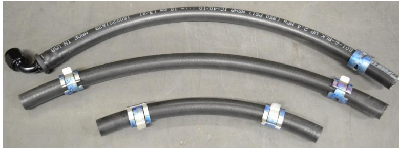
Hoses with factory clamps installed.
