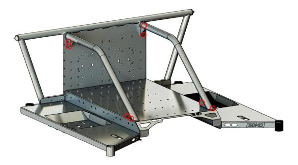
**6.** Use (2) 5/16" – 18 x 3/4" Grade 8 Hex head bolts, (4) 5/16" washers and (2) 5/16 – 18 Lock Nuts for each tie down mount. Bolt the mounts as pictured below. The mounts can be placed where needed on the Bed rack.
