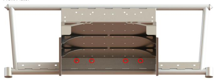
3. Align the Driver Side Plate next to the Front Plate and Floor Plate. There is a total of (7) 5/16" – 18 x 3/4" Grade 8 Hex head bolts that will be used on this side. (3) bolts will connect the Driver Side Plate and the Front Plate. The other (4) bolts will connect the Driver Side Plate and the Floor Plate. Be sure to use the 5/16" washers on both sides of the bolt.
