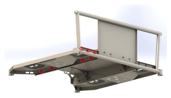
**5.** Align the Driver Support Tube with the Floor Plate and Front Plate as pictured. Insert (4) 3/8" – 16 x 3/4" Grade 8 Hex head bolts with 3/8" washers through the Driver Support Tube on the Front Plate and Floor Plate. Place 3/8" washers and thread 3/8" – 16 Lock Nuts onto the 3/8" Hex head bolts. Repeat this for the Passenger Support Tube.
