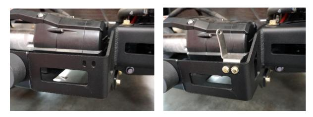
**3. Light Bar Install:** Mount the light bar to the driver side bracket using the Baja Designs supplied hardware. Support the bar and install the passenger side hardware. Align the bolts in the center of the slot and tighten.
