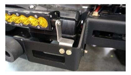
**4.** Center the light bar brackets in their mounting slots and tighten the supplied <sup>1</sup>/<sub>4</sub>" hardware locking the light bar in place.
