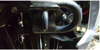
\*Note: If you have a TRD Pro or TRD Pro skid plate you need to add the provided spacers between the lower supports and winch mount using the included longer bolts.
