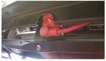
11. Mount the bumper skin to the factory mounts that are already bolted to the SDHQ winch mount. Make sure the Hawse or roller fairlead line up with your cutout, and adjust if necessary. Now is a good time to plug your sensors back into the wires before bolting the bumper back on the truck.
