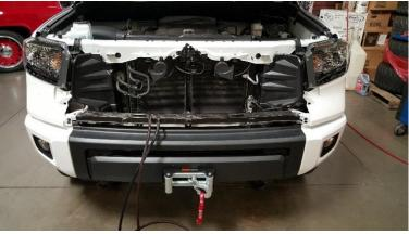
**14.** Install the 2 supplied lower support brackets. Bolt the front of the brackets to the mount using the supplied 7/16" hardware, and bolt the back of the brackets to the frame using the factory hardware through the tow hooks and the bracket. Some trimming of the plastic may be required.
