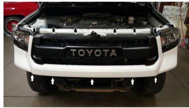
**13.** Install the bumper/winch mount assembly on the truck. Make sure you have at least 2 people to lift the heavy bumper and winch assembly. Level the bumper to match your truck and tighten the (8) 14mm nuts.
