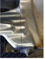
**10. 2014+ Models only.** Place the bumper skin on the mount and mark where the winch cables may come in contact with the factory bumper. Trim the sheet metal on bumper to clear as shown.
