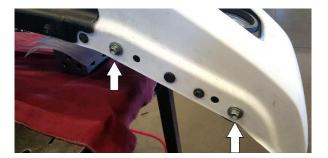
**4.** Next remove the 2 steel mounts from the factory aluminum mount.
