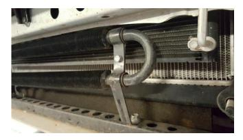
**9. 2010-2013 Models only.** Mark the inside edge of the lower sheet metal section of the factory bumper on both sides. Cut the sheet metal and remove the center section. Clean up all sharp edges on remaining sheet metal.
