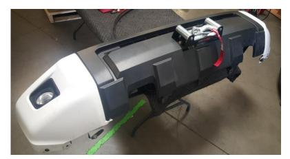
12. 2014+ Models only. Before installing the bumper on the truck, remove the grille by removing the (4) 10mm bolts, 2 plastic push clips and 5 lower clips. This will allow easier installation and routing of the cables.
