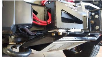
**15.** Wire your winch according to manufactures specifications. Secure all wiring so no damage can occur due to abrasion or pinching. Reinstall your grill with the factory clips and hardware (2014+ models only). If the Zeon Relocation kit was purchased, secure the wires as shown below with the loom clamps and tek screws.
