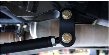
**18.** Measure the gap between the bump stop on the rear of the Traction Bars, and the bump plate on the Axle Mounts. It is recommended to have ~ 1/8" gap. If required, remove the 5/8" bolt and lower the Traction Bar. Install the supplied 1/8" and/or ½" aluminum spacers to reach the recommended gap and install the Traction Bar again.
