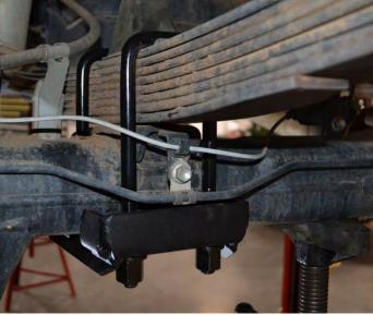
**14. Traction Bar Install.** Align (1) Traction Bar to the Driver Side Axle Mount. Install (1) 5/8" bolt, (2) washers and (1) locknut, securing the Traction bar to the Axle Mount.
