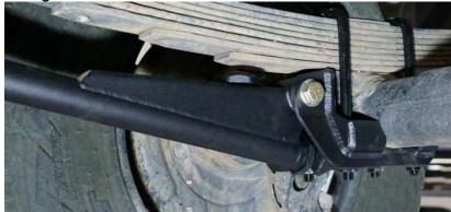
**17. Traction Bar Adjustment.** Install the wheels and set the truck on the ground. Adjust the heim such that the shackles are vertical from the ground. Tighten the Jam Nut against the Traction Bar to set the heims.
