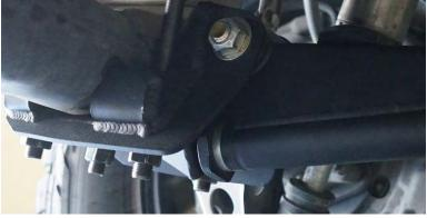
**19.** With the Traction Bar adjusted and all mounts installed, tight all 5/8" hardware. Torque the U-Bolts to 100-120 ft-lbs. Torque 5/8" hardware to 120 ft-lbs. Your SDHQ Built Traction Bar install is complete! Enjoy your increased traction.
