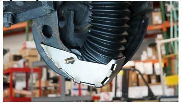
5. Next place the passenger capture plate into the lower mount from the inside of the mount and align with the rear bolt hole. When aligned, loosely thread in the supplied 3/8" hardware.
