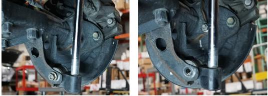
3. Cut the supplied shock boots for clearance as shown. Use soapy water to help slide the boot on the shock, as well as a second person to pull the shock away from the lower mount. Alternatively, remove the shock from the vehicle. Once cut, slide the larger opening over the lower RXT Shock Mount. Work the boot into place with the cut section towards the shock mounting bolt. Zip tie the boot to the top and bottom of the shock.
