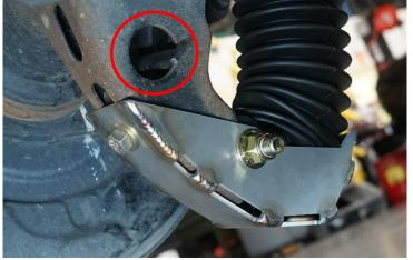
6. Repeat steps 2-5 for the driver side shock. Torque 3/8" hardware to 15 ft/lb. Lower the vehicle down to ride height and tighten the lower shock bolts to factory torque specs. Enjoy your new SDHQ Built Tundra Shock Guards!
