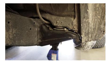
2. Place the Body Mount Cut Template against the body mount, centering the hole with the bolt as pictured. Sharpie around the template to mark what is needed to be cut. Use a Sawzall and the metal blade to cut the flat parts of the body mount. Use the grinder to finish cutting the body mount and clean up the cuts.
