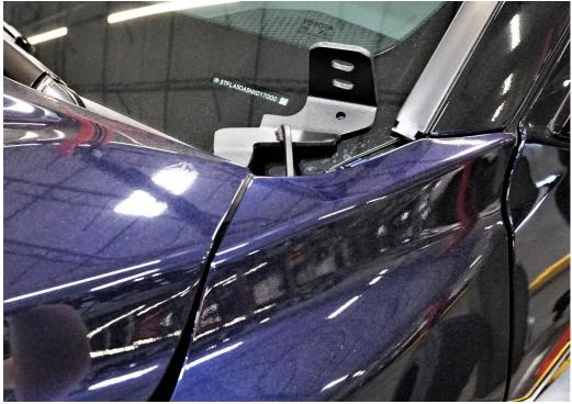
**5.** Completely remove the remaining hood hinge bolt and place the A-pillar over the holes. Start with the rear bolt hole and install the M8 Flange Head bolts into the frame. (**Note:** The silicone isolator can make starting the bolts difficult, you can use the A-pillar to move around the assembly in order to more easily start the bolts.)
