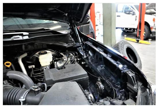
**3.** Starting on the Driver's side, prop your hood up and remove the rearmost hood hinge bolt located on the frame and loosen the front bolt using your 12mm socket. Leave the front bolt attached to the frame for now. The driver side hood hinge will have a washer line that will need to be unclipped
