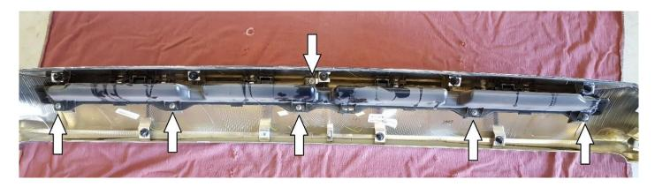
**3.** Using side cutters or a barrel sander, cut the outer top (2) clip mounts on both sides of the plastic as shown below. This cut is to ensure clearance of the light bar. Re-insert the (2) factory clips as shown below.
