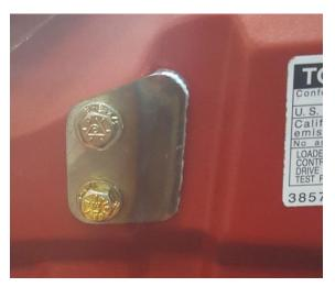
**10.** Use the provided  $\frac{1}{4}$ "-20 x  $\frac{1}{2}$ " bolts and flat washer to mount the light from the side.
