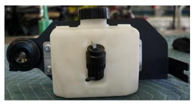
6. Wiring the Windshield Fluid Reservoir. Connect the grey connector on the supplied wiring harness to the factory windshield fluid pump connector as shown below. Run the wiring harness down the passenger fender to the firewall as shown below. Secure it to the factory harness using zip ties. The wiring harness will run behind/below the reservoir when installed.
