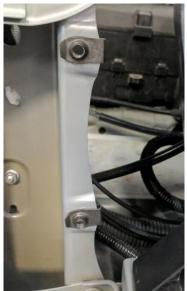
**4.** Place the Switch Pros Power Module and Mount over the Barrel Nuts and bolt into place with the  $\frac{1}{4}$ " - 20 x  $\frac{3}{4}$ " S.S Button Head bolts and  $\frac{1}{4}$ " S.S. washers as pictured. The Power Module can now be wired up.
