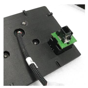
**4.** Once finished and wiring has been ran, install the panel in the reverse order as removed. The new panel is a tight fit, it may help to use your panel removal tool to guide the edges in place. Enjoy your new SDHQ Built Switch Pros RCR-Force-12 Overhead Console Mount!
