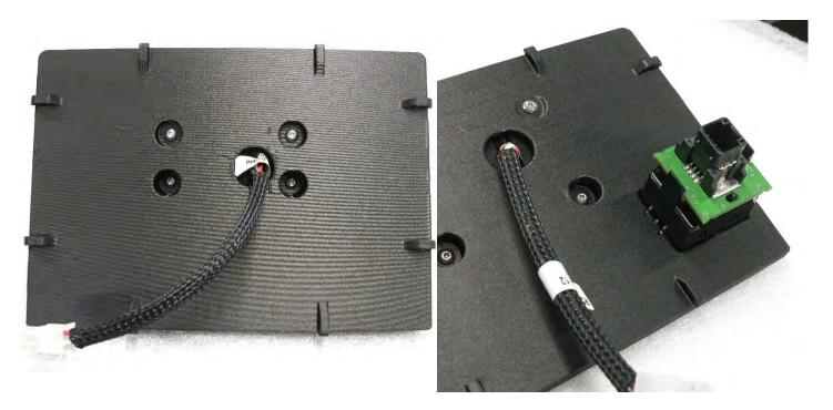
**4.** Once finished and wiring has been ran, install the panel in the reverse order as removed. The new panel is a tight fit, it may help to use your panel removal tool to guide the edges in place. Enjoy your new SDHQ Built Switch Pros 9100 Overhead Console Mount!
