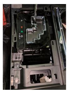
3. Once finished and wiring has been ran, install the panel in the reverse order as removed.
