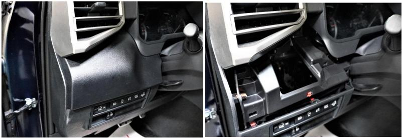
3. Position and secure with tape, your bare keypad mount on the dash trim piece as pictured. Drill a 1/8" pilot hole into the panel using each of your mounts bolt holes as a guide and another pilot hole in the center opening of the bare mount towards the front of the panel. Remove the keypad mount and re-drill the (4) bolt holes with your 5/32" drill bit and use your step drill bit to drill your center hole to <sup>3</sup>/<sub>4</sub>" for the wire harness.
