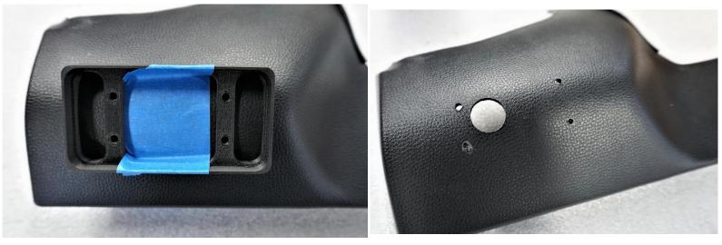
**4.** Turn the panel over and trim any ribs that would keep the backers from mounting flat against the back side.
