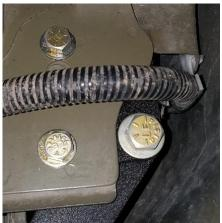
**4.** Remove the factory lower bedside supports with a 10mm socket or wrench. Install the new Fender Support Replacement pieces with the curved section sweeping toward the back of the truck using the provided ¼" hardware. Install the Lower Mounts to the factory receiver hitch using factory bolts as shown.
