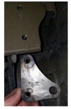
**3.** Slide the Main Upright through the top of the tail light opening. Loosely bolt the upper bolt through the upright, the factory sheet metal, and into the Upper Bolt Puck using the 7/16" bolt and washer. Be careful not to drop the puck while installing. It is difficult to recover if dropped. Thread Lower Pivot Bracket and the Main Upright together with the ½" bolt and washer.
