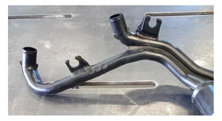
**5.** Insert the 2 aluminum adapters in the factory rubber intake hoses and secure with the factory clamps. Remove the top plastic clip holing the front inner rubber flap.
