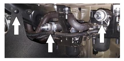
**6.** Run the 2 lines from the engine compartment down and through the inner fender opening. The longer line attaches to the farthest pump from the frame, and the short line with the 90° fitting to the closest. Run the lines behind the power steering reservoir hose so the power steering pulley does not interfere with the lines.
