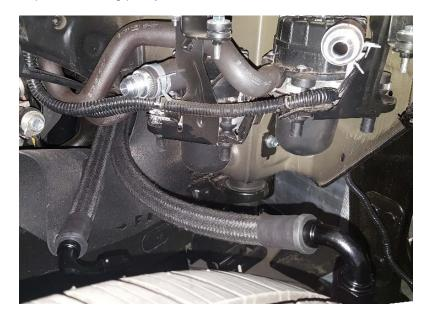
7. Connect the 2 lines and re-attach the rubber flap.
