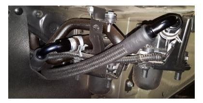
8. In the engine compartment, run the 2 lines behind the windshield washer bottle.
