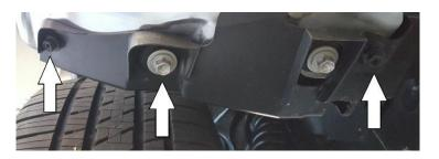
**3.** Remove the (3) 10mm bolts in the front of the inner fender. Remove all the factory push clips on the side. Using a panel tool and a pick, carefully pry up and bring the 2 side pins together to release. Try not to damage these clips because they will be used to reinstall the factory inner fender. Now remove the inner fender.
