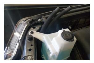
**9.** Use the provided edge clip zip tie and attach to the fender inner sheet metal between the washer bottle and air box. Install the provided 2 piece clamp, hose clamps, and 2 filters. Fasten the upper line to the edge clip with the zip tie and trim the excess.
