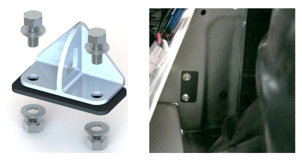
5. Installing the SDHQ Battery Hold Down. Group 34/34R Batteries will use the 8" J-Hook, all others will use the 9" J-Hooks. Place the SDHQ Billet Aluminum Adapters through the SDHQ Battery Hold Down. Insert the J-Hooks through the Adapters and thread on the ¼" – 20 Flange Nuts onto the J-Hooks. Place the SDHQ Battery Hold Down on the battery. While tightening the ¼" nuts, hook the J-Hooks to the factory tie down and SDHQ Tie Down.
