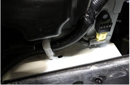
**3. Drilling.** Align the Main Tie down with the panel clip slot from Step 2 and parallel to the battery. Mark the other hole in the fender to be drilled. Remove the Main Tie Down. Drill a hole through the mark and the slot. Deburr if necessary.
