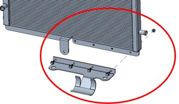
**5.** Prepare the SDHQ Water Pump Relocation Bracket. Insert the (4) #10-24 Nut Clips onto the flange of the intercooler, be sure to line them up with the predrilled holes. Install the Aeromotive clamp onto the flange of the relocation bracket, with the nut side facing out, using the (2)  $\frac{1}{4}$ "-20 bolts, (4)  $\frac{1}{4}$ " washers and (2)  $\frac{1}{4}$ "-20 Top Lock nuts, leave the hardware loose to aid in positioning the water pump during installation.
