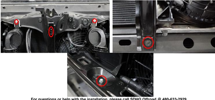
For questions or help with the installation, please call SDHQ Offroad @ 480-633-2929 Mon.–Fri. 8:00am–5:30pm and Sat. 8:00am–3:30pm Arizona Time. www.sdhqoffroad.com Page 4 of 4 **3.** Disconnect and unbolt the intercooler fan and set aside. Next, remove and discard the 2 clamps holding the water pump to the Harrop bracket, pictured below. Secure the water pump out of the way for now.
