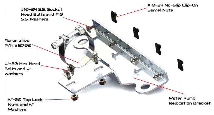
**1.** If you have previously installed the Harrop Supercharger TVS2650 Kit, you will need to unbolt the intercooler enough to reach the nuts holding the original water pump bracket to the intercooler. If you are installing the supercharger kit and the SDHQ Built Hidden Winch Mount concurrently then you can skip to Step 5.
