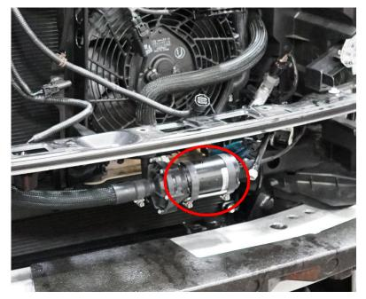
**4.** Now the intercooler will be able to move enough to get to the (4) 10mm nuts out from behind the intercooler. Carefully pull the bottom of the intercooler towards you and remove the (4) 10mm nuts and bolts, bolt locations pictured below. Now, you can remove and discard the original Harrop water pump bracket.
