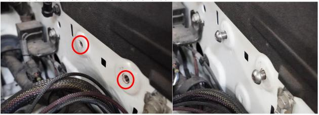
**3.** Slide the assembled mount and Switch Pros Power Module onto the bolts and tighten. Then finish wiring and enjoy your **SDHQ** Switch Pros Power Module Mount!
