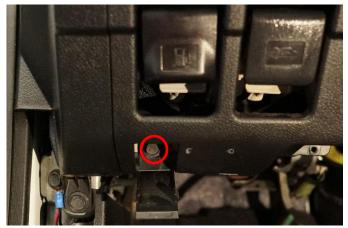
3. Now remove the panel below the gas and hood release mechanism and disconnect all connections. Take note of where the (2) rear tabs are located for assembly later.
