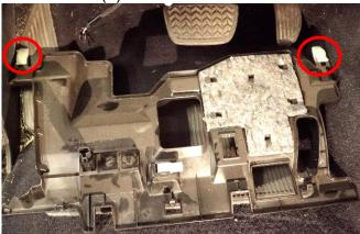
4. Now pry off the panel underneath the steering column and disconnect any electrical connections and take note of where each connection goes. Start from the bottom and work towards the top and pull out.
