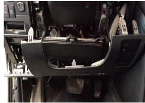
**6. Mounting the Switch Pros.** Now that the panel is removed, pop out the factory switch cluster to prepare for the install of the Switch Pros. Any factory switches in this panel will need to be relocated.
