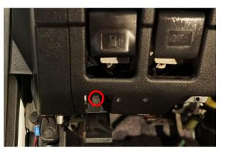
**4.** Now remove the panel below the gas and hood release mechanism and disconnect all connections. Take note of where the (2) rear tabs are located for assembly later.
