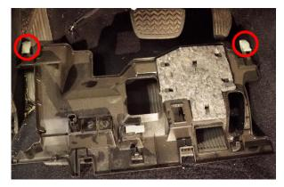
5. Now pry off the panel underneath the steering column and disconnect any electrical connections and take note of where each connection goes. Start from the bottom and work towards the top and pull out.
