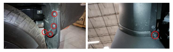
**3.** Using a plastic clip tool, 10mm socket and a ratchet remove the fender flare from the driver side rear quarter panel.
