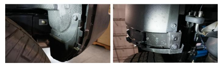
5. Using a plastic clip tool, 10mm socket and a ratchet remove the wheel liner from the rear driver side wheel well.
