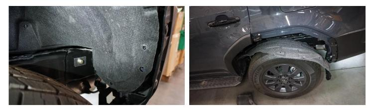
6. Using a 12mm socket and a ratchet remove the bolt retaining the second fuel neck support.
