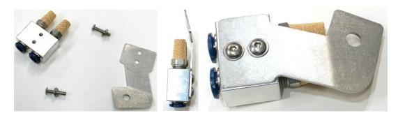
9. Using a 12mm socket and a ratchet install the filter mount onto the second fuel neck support.
