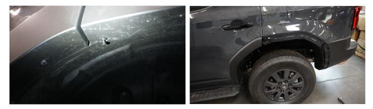
**4.** Using a plastic clip tool, 10mm socket and a ratchet remove the plastic liner portion from the rear of the driver side rear wheel well.
