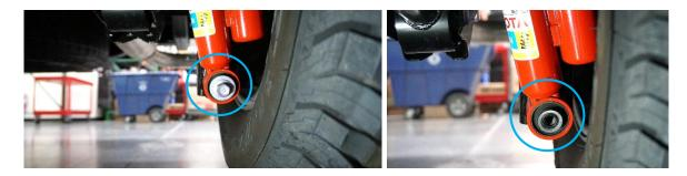
3. Slide (1) Shock Guard over the driver side rear shock and shock mount as shown. Place (1) M12 bolt through the Bolt Guard and put Red Loctite on the threads then start threading into the shock mount. Using a 17mm socket tighten the M12 bolt but leave loose.
