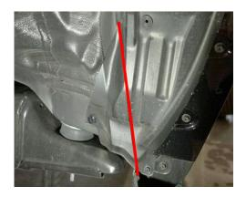
3. Cutting the mounts. Place the body mount template against the body mount and outline. Outline along the template following the red line shown below. Be sure to follow the red line exactly. Use a Sawzall and a metal blade to cut the flat parts of the body mount. Use a cut off wheel to finish trimming the body mount and cleaning up the metal. Some excess material may be cut off of the bottom body mount washer if the body mount chop plate hits the washer.
