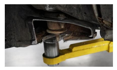
**4. Installing the chop plate.** Verify fitment of the body mount plate. If the plate sits flush against the chopped body mount, tack in place. If it does not, cut what needs to be trimmed and then tack. If there are gaps due to over-cutting, fill in with weld. Once the placement is verified, weld the mount into place. Paint over any bare metal once complete to prevent any rust.
