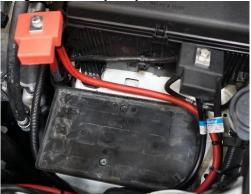
4. Place the mount into the battery tray with the REDARC/PM facing the passenger side of the vehicle. Replace your battery on top of the mount, adjusting the position as desired.
