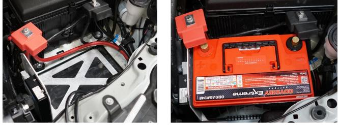
5. Reinstall your battery terminals and tie down. The battery recharger can now be wired according to REDARC installation instructions. Enjoy your new SDHQ Built REDARC/Switch Pros Battery Mount!
