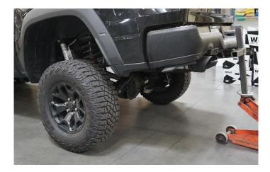
**2.** Loosen your driver side lower shock bolt using a 22mm wrench and socket. Remove the shock bolt and angle the shock out of the mount slightly as shown.
