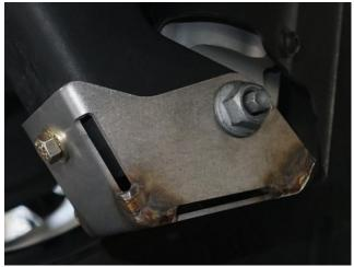
**5.** Repeat steps 2-4 for the other shock and tighten all 3/8" hardware. Lower the vehicle down to the ground and tighten the lower shock bolts to factory torque specs. Enjoy your new SDHQ TRX Shock Guards!
