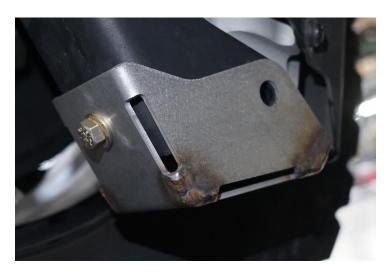
**4.** Check alignment of the driver shock eye to the lower mount hole, lifting the vehicle if the shock eye is low and lowering the vehicle if it is too high. Once aligned slide the shock guard up and reuse the factory shock bolt and nut, threading it on loosely.
