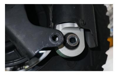
**3.** Align the shock guard onto the lower mount and loosely thread the supplied 3/8" bolt through slot on the shock mount using a washer on either side.
