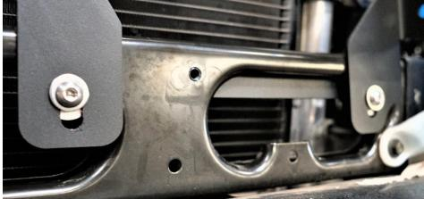
**13.** Before tightening all the hardware, take your straight edge and level, then set them in a slot and level your mounts with your truck side to side. Then tighten all hardware.
