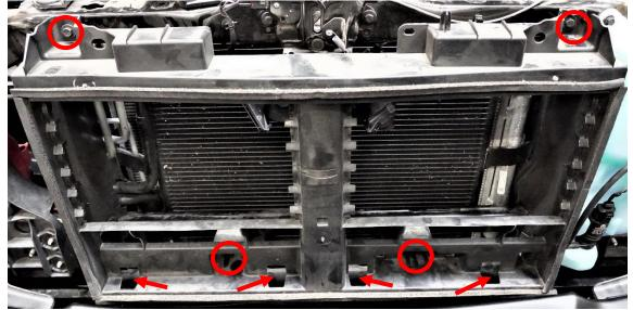
7. <u>Removing Active Grill Shutter motor.</u> First locate the plastic cover on the front of the shutter frame and slide it out of its spot as shown. Then using your panel removal tool, pry the outside edge of the frame to release the outside of the (2) shutters directly connected to the motor. Now unclip the (12) tabs holding the shutters to the inside of the frame and discard the cover. Fully remove the (2) shutters directly connected to the motor from the frame by pulling toward you.
