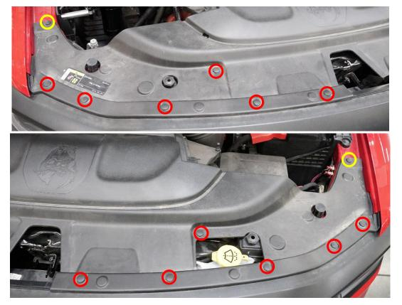
2. Next remove the (8) 10mm bolts and (2) clips holding in the upper trim and upper grille assembly. Gently pull the upper trim towards the front of the vehicle and set aside.
