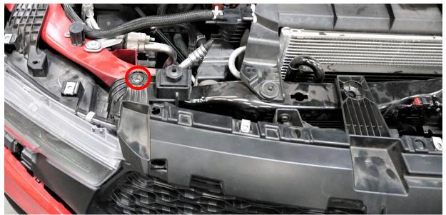
5. Unclip any connectors behind the grille, remove grille and set aside.
