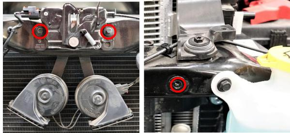
12. Now place both Lower Backer Mounts into the lower core support with the weld nuts facing toward the radiator and bolt them through Mounts on A & B on the Driver and Passenger sides. (Note: Be sure to push the backer up into the core support as much as possible when installing)
