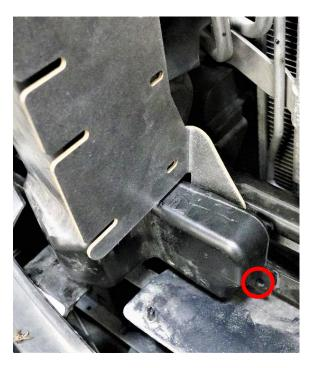
12. <u>Installing the Brackets</u>. Start by loosening the (2) 10mm bolts holding on the hood latch, then carefully bend the bracket holding both horns backwards, toward the radiator. Now, slide the Driver and Passenger Side Mount B into place **behind** the hood latch and snug the hood latch bolts up so that the mounts won't fall. Similarly, using the supplied M6 bolts and washers, bolt the Driver and Passenger Mount A into the upper bolt holes on the core support.
