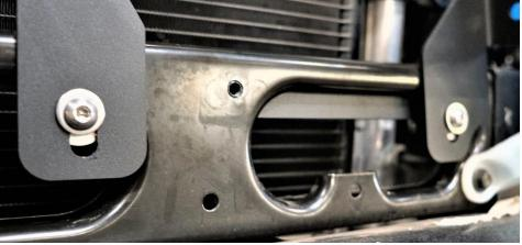
**14.** Before tightening all the hardware, take your straight edge and level, then set them in a slot and level your mounts with your truck side to side. Then tighten all hardware.
