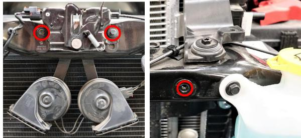
12. Now place both Lower Backer Mounts into the lower core support with the weld nuts facing toward the radiator and bolt them through Mounts on A & B on the Driver and Passenger sides. (Note: Be sure to push the backer up into the core support as much as possible when installing)
