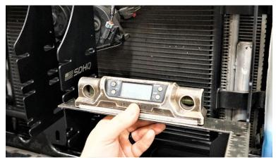
14. Install Light Bars. If you are mounting an OnX6 10" light bar then you need to place ¼" washers between the light and the mount. Place your lights in the appropriate slots as seen on Page 4, some models can run (4) lights per truck (see picture below).
