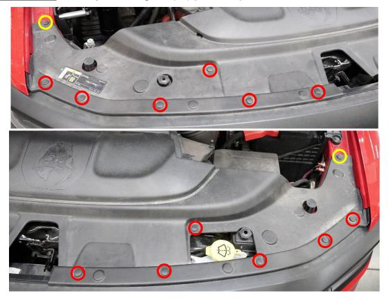
2. Next remove the (8) 10mm bolts and (2) clips holding in the upper trim and upper grille assembly. Gently pull the upper trim towards the front of the vehicle and set aside.
