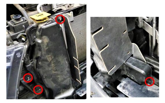
11. <u>Installing the Brackets</u>. Start by loosening the (2) 10mm bolts holding on the hood latch, then carefully bend the bracket holding both horns backward toward the radiator. Now, slide the Driver and Passenger Side Mount B into place **behind** the hood latch and snug the hood latch bolts up so that the mounts won't fall. Similarly, using the supplied M6 bolts and washers, bolt the Driver and Passenger Mount A into the upper bolt holes on the core support.
