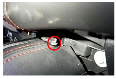
**4.** Use your trim tool to unclip the center console panel and lift until you can see the T20 retainer bolt that holds the shifter in place. Using your long extension, loosen and remove the retainer bolt from the shifter. **Note:** Do **NOT** drop the retainer bolt into the shifter assembly
