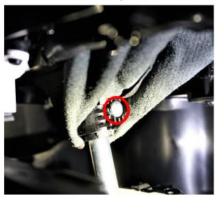
**5.** Unclip the electrical connector in the panel and remove from the vehicle.
