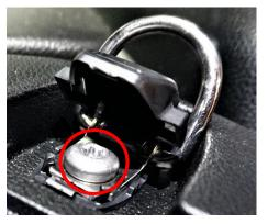
**3.** Remove the (2) remaining 10mm bolts holding the storage bin to the truck. Leave bin in place
