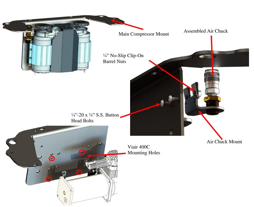
Note: In order to mount the Viair 400C you will need to remove the brackets attached to the compressor and move them to position shown. For the bracket closer to the pump, you will need to use the supplied M5 hardware to mount the bracket securely
