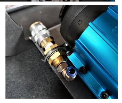
7. Pause install now to wire your compressor, refer to the ARB wiring instructions to properly wire your air compressor. Note: We recommend that when you drill a hole for the wire harness in the storage bin, that you de-pin the connector to minimize the size of the hole.
