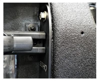
**6.** Use your 21mm socket to remove the upper (2) bolts that secure the trailer hitch to the frame. Note that the longer bolt goes toward the rear of the truck.
