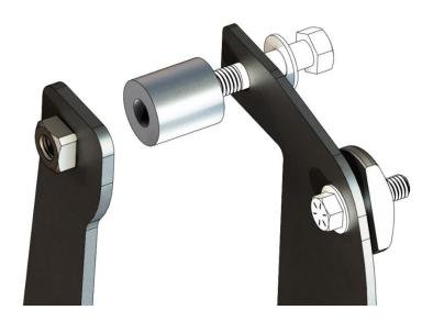
**11.** Take your Frame Mount and connect it to the frame using the (2) frame bolts removed earlier, note that the Frame Mount is offset and the longer side points towards the back of the truck as shown. Tighten frame bolts to 110 ft/lbs (+/- 5ft/lbs).
