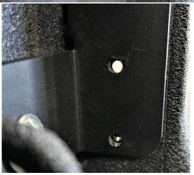
**9.** Once both holes are drilled, assemble the SDHQ Billet Tie Down with the 5/16" x 1-1/2" hardware using the lock nuts on the inside of the fender as shown. The hardware supplied with
