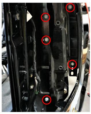
**5.** Some trucks come equipped with tie down rails, you will need to remove the (8) 10mm bolts per side holding the rail to the bed to remove the rail for install of the bedside supports. Use your 4mm allen head socket to unbolt the end cap on the tailgate side of the tie down rail, the cap will not fit with the installed bed side support.
