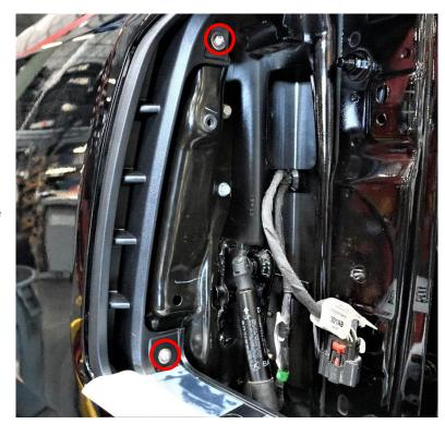
**4.** Remove the (5) 10mm bolts from the sheet metal that has been exposed after removing the tail light and tail light vent bezel. Set aside the sheet metal piece.
