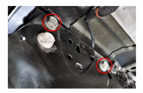
7. Start your install by sliding the Bedside Upright through the opening in the bed and installing a 7/16" bolt / washer into the top hole and bolting to the Trimmed Upper Bracket. The Trimmed Upper Bracket will sit in the opening visible from the top of the bed side, place the bracket in through the tail light opening as shown.
