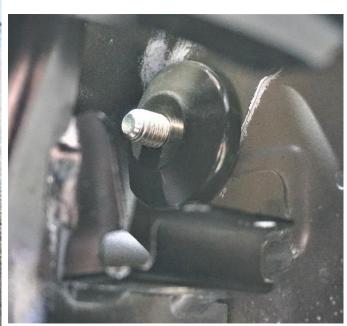
8. Now place the ½"-13 carriage bolt into the square opening in the Bedside Upright and place the Fender Pivot on the other side of the bolt, install the ½"-13 nut/washer and tighten the all the hardware installed up to this point. Using the supplied drill bit, drill through the bed using the (2) holes in the Bedside Upright as a template. (Note: you may have to remove/reinstall the Bedside Upright once the holes are drilled to debur them and paint the holes to prevent rust from forming)
