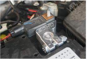
**13. Installing the Negative Distribution Block:** Assemble the negative distribution block as shown in the diagrams on page 4. Remove the driver fender support bar using a 13mm socket on the nut and bolt.
