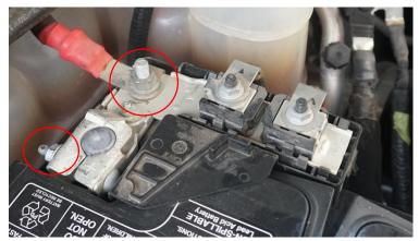
8. Passenger Side Positive Install Continued: Unclip the bus bar from the plastic base so it can be trimmed. Using flush cuts/pliers trim the plastic as shown below. Be sure not to trim off the back clip shown in blue. When complete snap the bus bar back into the bottom housing.
