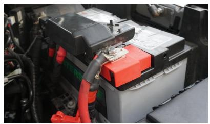
7. Passenger Side Positive Install: Begin by unclipping the plastic cover on the positive terminal followed by the 13mm and 10mm holding the terminal to the bus bar and batteries. Set the terminal aside to be replaced.
