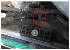
**10.** Passenger Side Positive Install Continued: Attach all necessary accessories to the positive terminal and then install the SDHQ red terminal boot. Install the bus bar and positive wire to the top 5/16" bolt hole on the terminal and replace the plastic cover.
