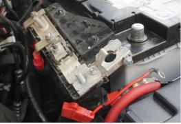
**4. Driver Side Positive Install Continued:** Next trim the bottom of the cover using some flush cuts as shown below. When trimmed snap the bus bar back into the plastic housing. Be sure to not trim off the front clip shown in blue below.
