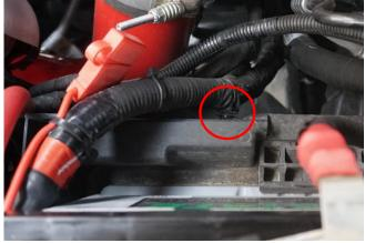
6. Driver Side Positive Install Continued: Attach all necessary accessories to the positive terminal and then install the SDHQ red terminal boot. Install the bus bar and positive wire to the top 5/16" bolt hole on the terminal and replace the plastic cover.
