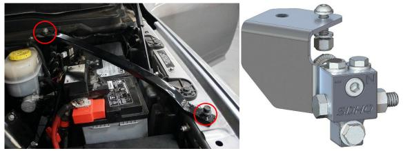
**9. Installing the Negative Distribution Block Continued:** Attach the distribution block to the mount using the M8 socket head bolt and M8 flange head nut as shown. Then install the mount on the fender support stud rotating it under the plastic cowling. Replace the fender support over the mount and secure using the supplied ½" hardware.
