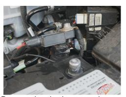
3. **Driver Side Positive Install:** Remove the plastic strap going across the battery and set it aside. Remove the driver's side positive terminal using a 12mm, 10mm and 7mm socket. Once all bolts are removed open the plastic cover and unclip the bus bar from the plastic housing. Remove the positive terminal and factory red terminal boot and set them aside.
