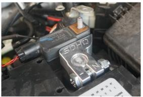
8. Installing the Negative Distribution Block: Assemble the negative distribution block as shown in the diagrams on page 4. Remove the driver fender support bar using a 13mm socket on the nut and bolt.
