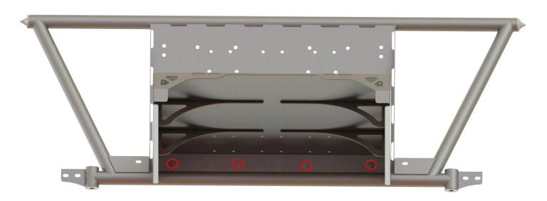
3. Align the Driver Side Plate next to the Front Plate and Floor Plate. There is a total of (7) 5/16" – 18 x 3/4" Grade 8 Hex head bolts that will be used on this side. (3) bolts will connect the Driver Side Plate and the Front Plate. The other (4) bolts will connect the Driver Side Plate and the Floor Plate. Be sure to use the 5/16" washers on both sides of the bolt.
