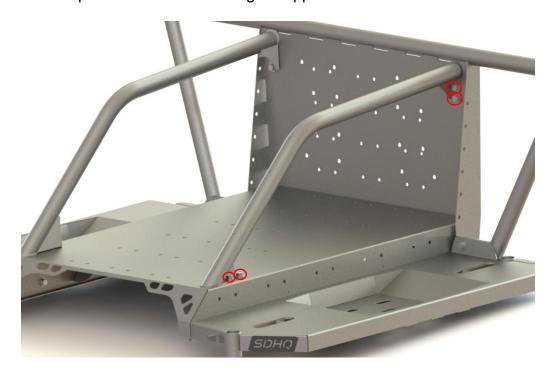
**6.** Use (2) 5/16" – 18 x 3/4" Grade 8 Hex head bolts, (4) 5/16" washers and (2) 5/16 – 18 Lock Nuts for each tie down mount. Bolt the mounts as pictured below. The mounts can be placed where needed on the Bed rack.
