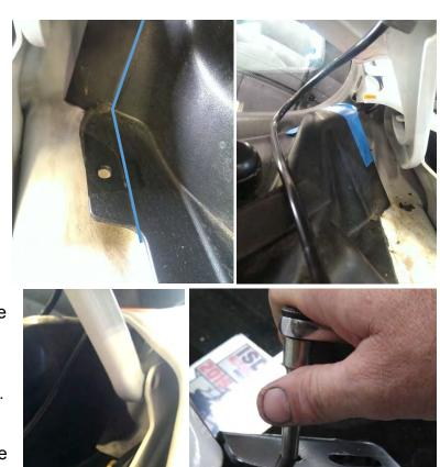
directly above the top fender bolt, simply install your 10mm socket on the head of the bolt and feed your ½" drive extension through provided hole in order to properly tighten. **Repeat Step 8 on Passenger side**
