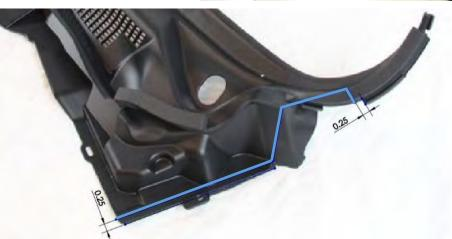
**Step 5:** Using the same method from step 4, remove the tab off of the passenger side plastic cowl and clean up any burrs or sharp edges.
