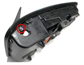
8. Run all necessary wiring before continuing the install. Connect all factory wire connectors to the panel and the switch pros harness to the keypad. Snap the panel back into the roof and reinstall the (2) 8mm bolts taken off from step 2. You can now close your new switch pro mount. Enjoy your SDHQ 3D Printed Sunglass Key Pad Conversion mount!
