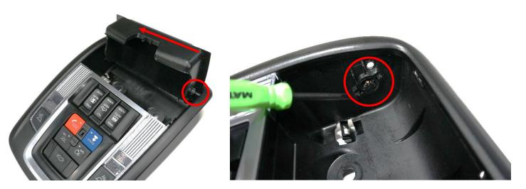
**4.** Install your Switch Pros keypad into the mount and secure it using the supplied (4) #6 screws. Next slide the (2) #8 nuts into the keypad mount with the washers facing in.
