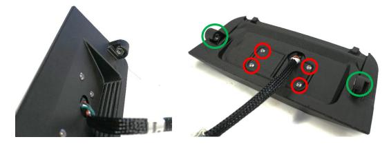
5. A <sup>3</sup>/<sub>4</sub>" hole will need to be drilled in the panel for the wiring harness to pass through. Mark a center dot on the angled portion on the back of the mount. Using a <sup>3</sup>/<sub>4</sub>" step bit, drill out the hole so that the electrical connector will fit the pass through.
