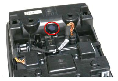
6. Now install the keypad mount into the panel starting with the sharp corners. With the mount half installed, pass the wire connector through the previously drilled hole. Do not snap the front of the mount into the panel yet, this will be done at the end of your install.
