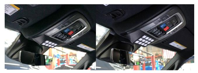
**9.** If needed, you can reopen your switch pro mount by inserting a plastic pry tool between the rear panel gap of the mount. Pop the panel open to access the 8mm bolts.
