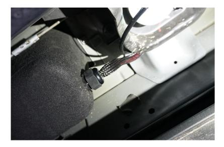
**3.** Attach a 1/4" Eyelet to the ground wire previously separated from the extension harness and heat shrink over the loom and eyelet. Using a supplied 1/4"-20 3/4" bolt, nut and washers secure the ground wire to the chassis on the body mount as shown.
