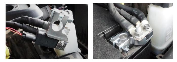
7. Installing the Positive Terminal. Double check that all connections are secure and that no wires were left disconnected. Using the supplied 8" zip ties, attach the negative wire along the run of factory negative wires leaving the little bit of slack on the distribution mount side. Routing shown on the next page.
