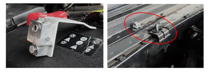
**4.** Install the mount over the stud and under the rear bolt. Tighten the front 10mm nut first then the rear 10mm bolt. Install the 25" negative cable to the D2 using the 3/8" bolt and leave the slack looped by the mount for now.
