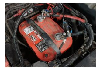
2. Disconnect the negative terminal from the battery and completely remove the 10mm nut. Then disconnect the negative wires from the terminal that can be removed using a 10mm socket.
