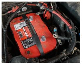
5. Installing the Positive Terminal. Install the SDHQ Terminal on the corresponding battery stud with a battery washer underneath. Lightly tap on the top of the terminal using a rubber mallet to set it on the battery post. Tighten the 5/16" Battery Bolt and Nut, using ½" wrench on both to prevent damaging the battery post. Connect all accessories to the terminal and then place the red battery cover on top. Connect the main power line to the top of the terminal.
