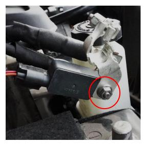
**3.** Installing the Negative Block. Assemble the distribution block with all hardware other than the 3/8" through bolt. Attach it to the mount using the M8 socket head bolt and M8 flange head nut as shown. Then remove the 10mm nut and washer off the shown fire wall stud second from the passenger side. Next loosen then 10mm bolt behind the nut such that the distribution mount can slide under.
